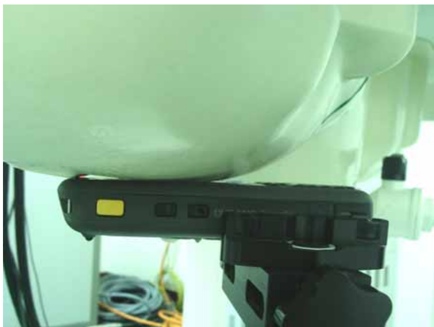
DUT with Battery 1 - Right Cheek
