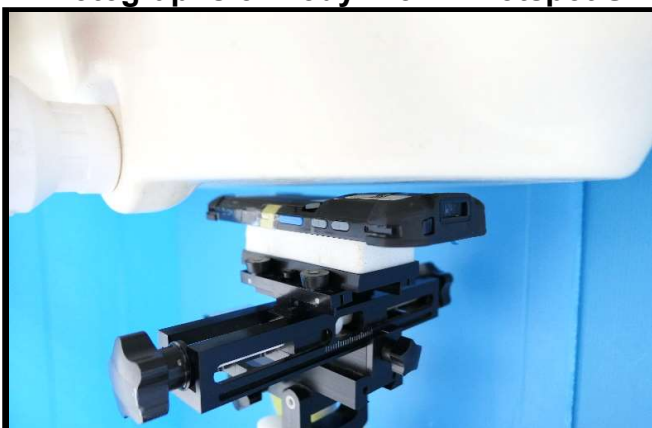
Rear Face of EUT Tested at 5 mm
