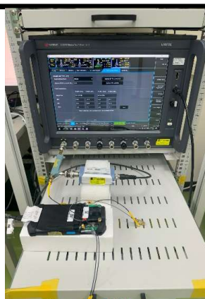
Setup for Conducted Power Test (for 5GNR SA)
