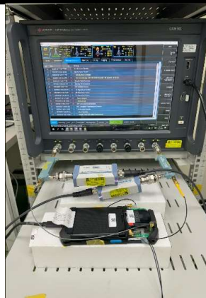
Setup for Conducted Power Test (for ENDC)
