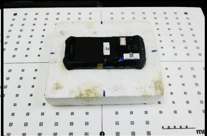
Rear Face of EUT Tested at 0 mm
