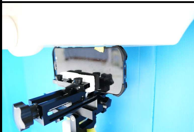
Right Side of EUT Tested at 0 mm
