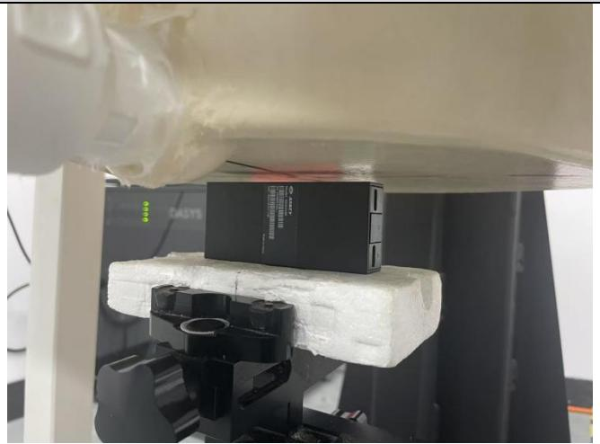
A photograph showing the right side of the EUT under the cylindrical probe. The probe is positioned to the left of the EUT, and the EUT is mounted on a black base with a white foam block. The probe is in contact with the top of the EUT. |
