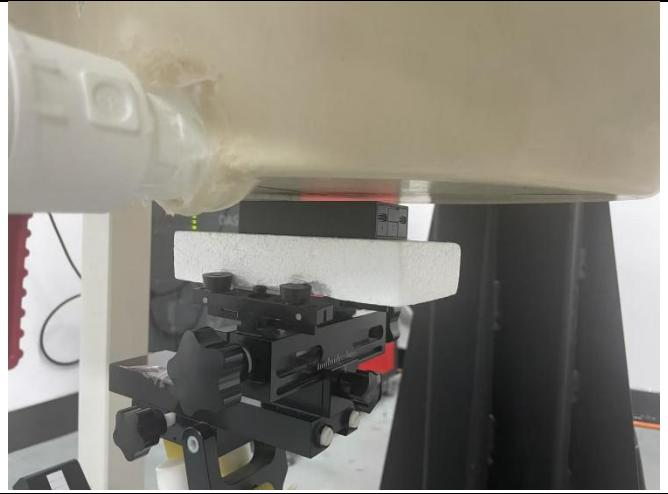
A photograph showing the back side of the EUT under the cylindrical probe. The probe is positioned to the left of the EUT, and the EUT is mounted on a black base with a white foam block. The probe is in contact with the top of the EUT.   |
