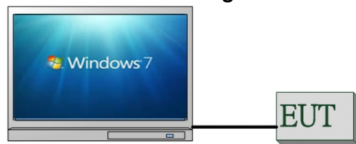
Fig. 2-3 Conducted (AC powerline) Emission Configuration
