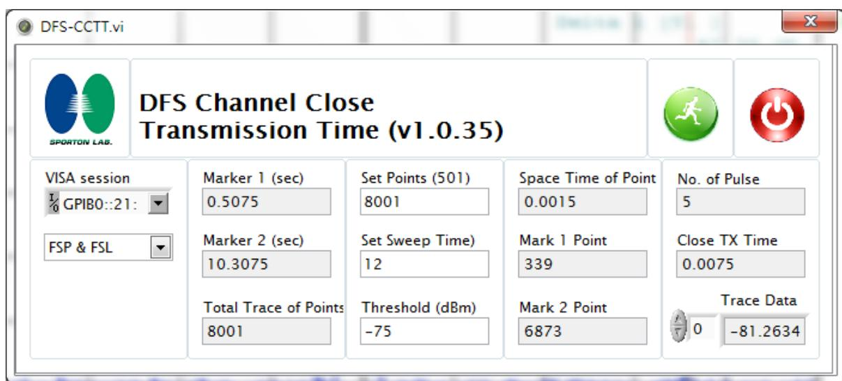
Radar #1 Channel Closing Transmission Time is comprised of 200 ms starting at the beginning of the Channel Move Time plus 0ms intermittent control signals of 9.8 sec period
