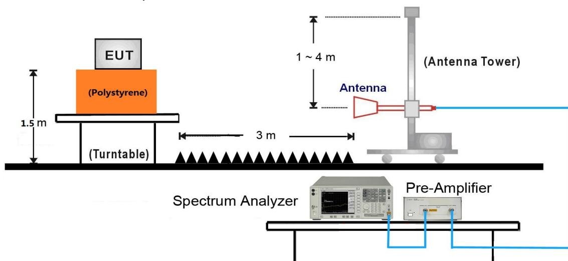
18GHz ~ 25GHz Test Setup:
