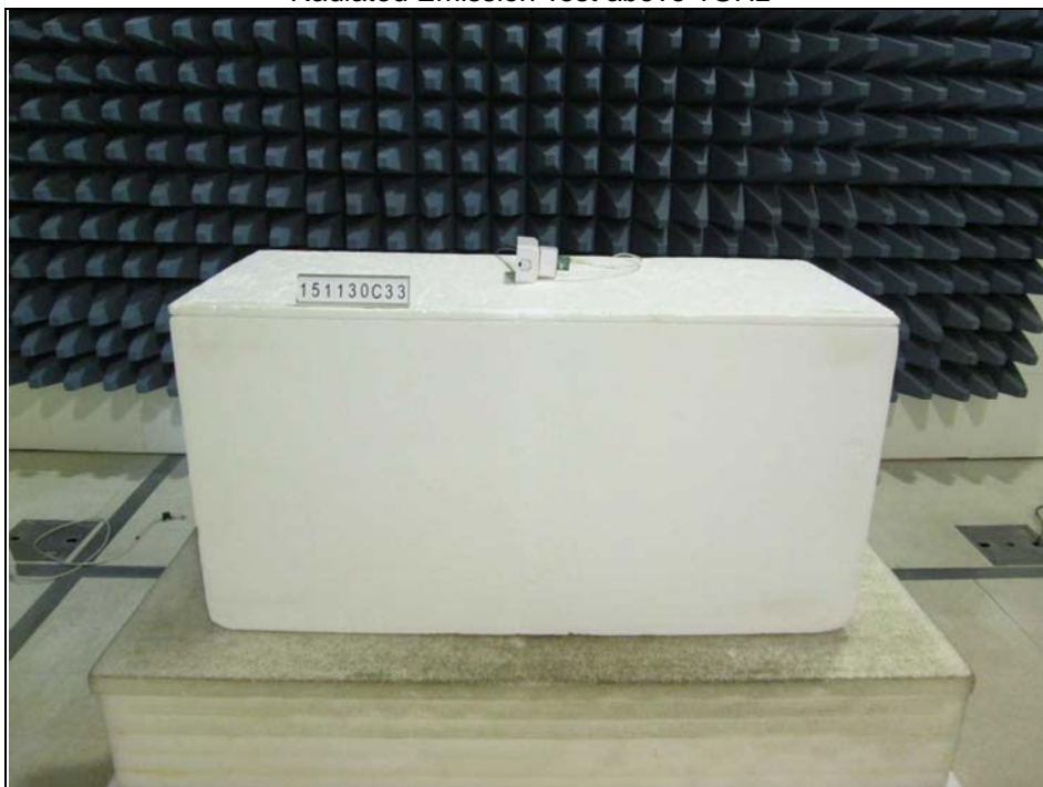
Radiated Emission Test above 1GHz
