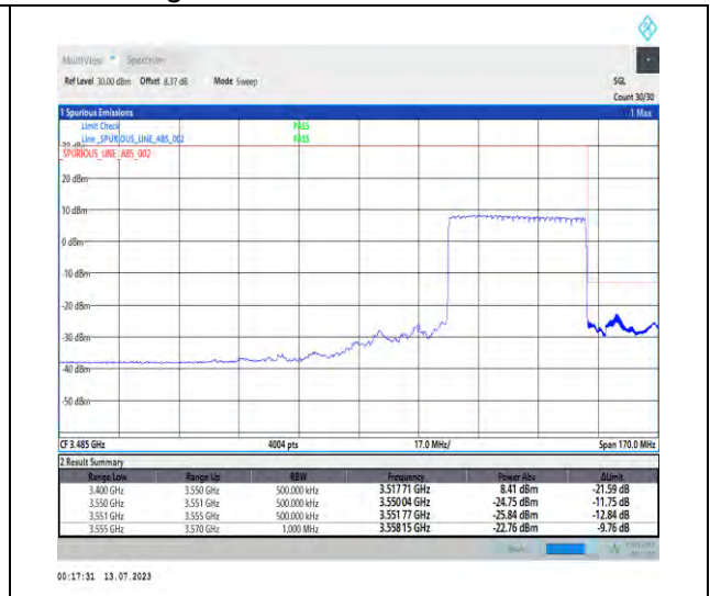
1-N77-3450-3550-PC1.5-30-40-H-3-DFT-PI2BPSK-Outer_Full-100@0-Ant3-1--PASS-see graph
