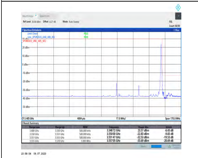
1-N77-3450-3550-PC1.5-30-50-H-5-CP-QPSK-Edge_1RB_Right-1@132-Ant3-1--PASS-see graph
