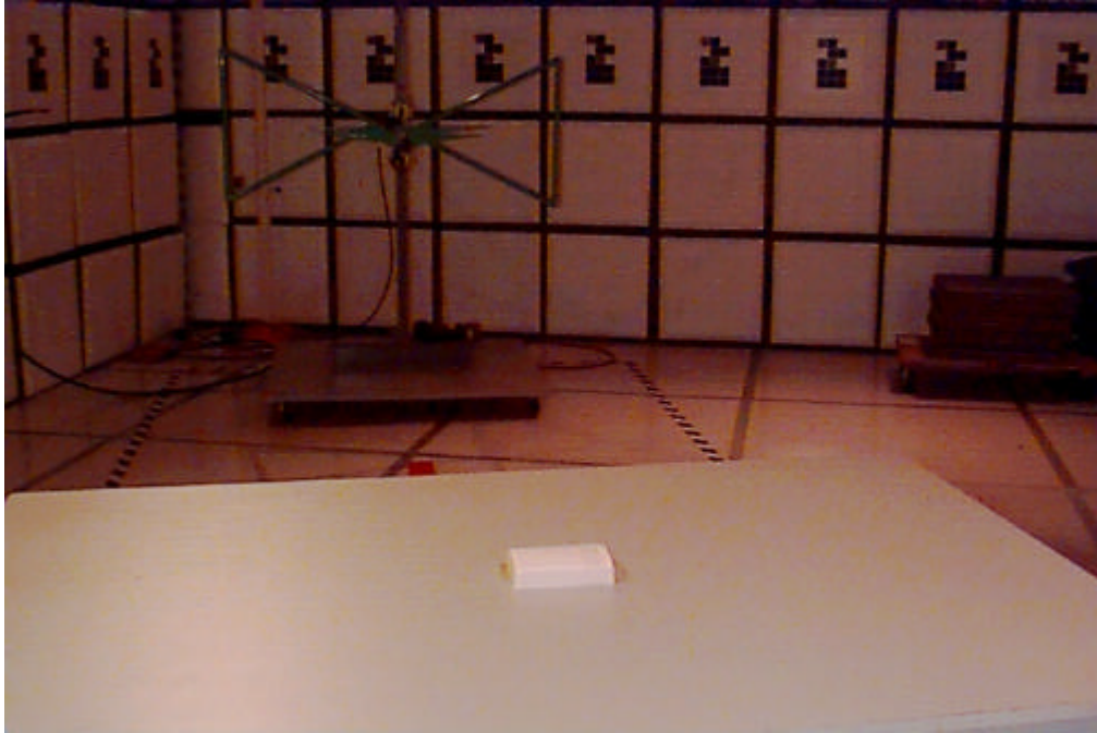
Radiated Emission Test Set-up – Receiver
