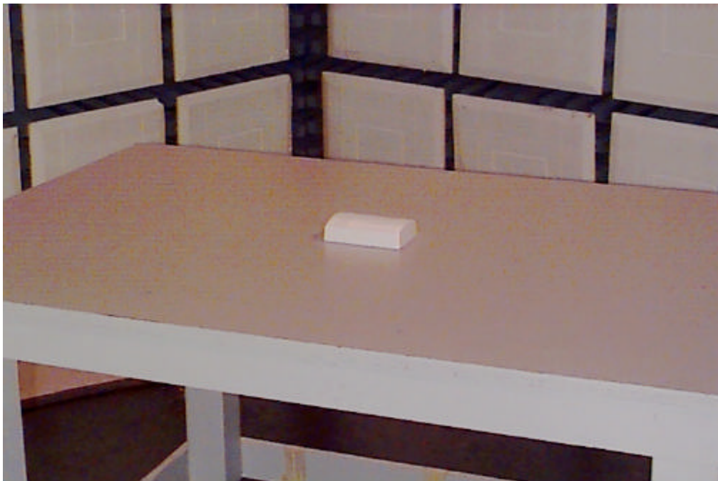
Radiated Emission Test Set-up – Receiver
