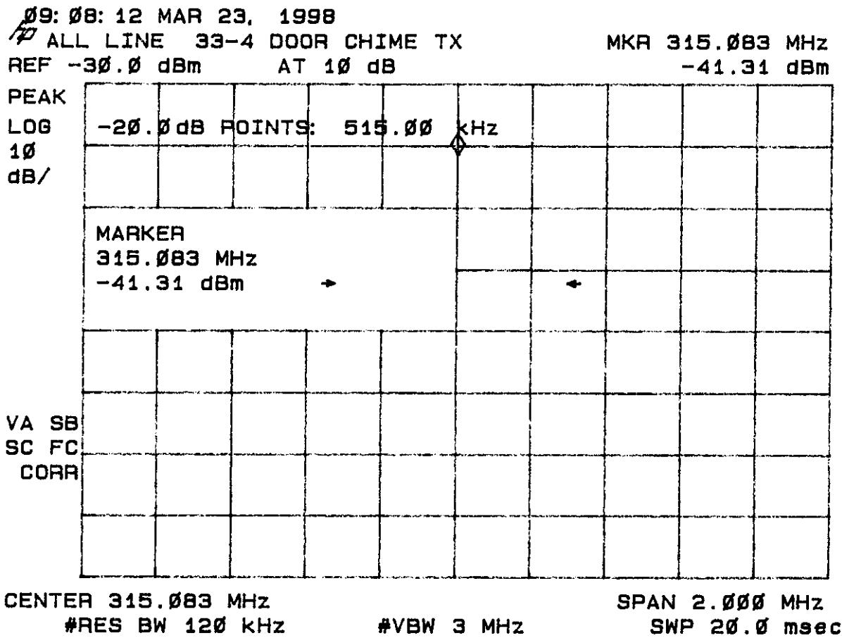
**Frequency Tolerance of Carrier Signal (47 CFR 15.231d)**
