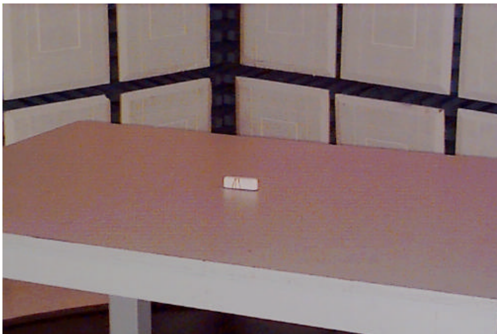
Radiated Emission Test Set-up – Transmitter
