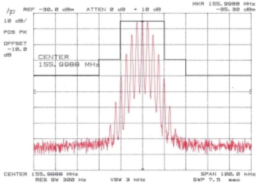
Occupied Bandwidth Low Power (5W); Wide Bandwidth (25KHz); 156MHz Plot - F3E
