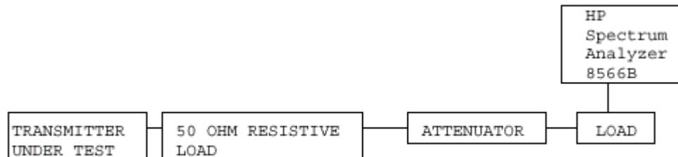
**METHOD OF MEASUREMENT:** The procedure used was the TIA/EIA-603-A STANDARD without any exceptions. An audio generator is connected to EUT through a dummy microphone circuit and the output of the transmitter is then connected to a standard load to a pre-selected filter of the spectrum analyzer. The spectrum is scanned from 30 MHz to a minimum of the tenth harmonic of the fundamental using a HP model 8566B spectrum analyzer.
