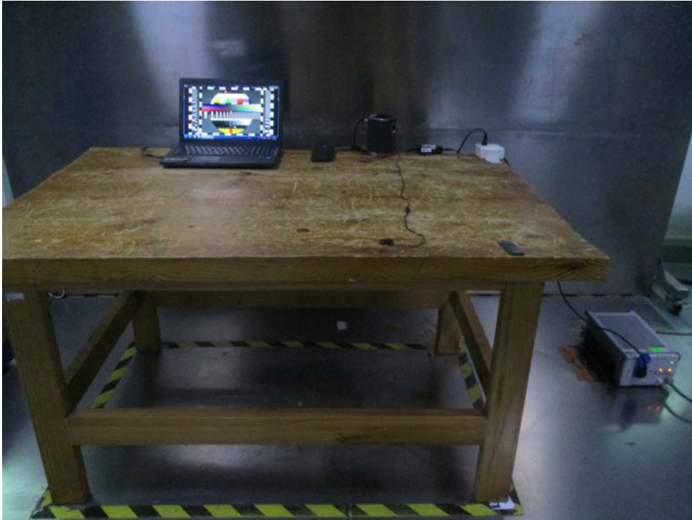
Conducted Emissions- side View
