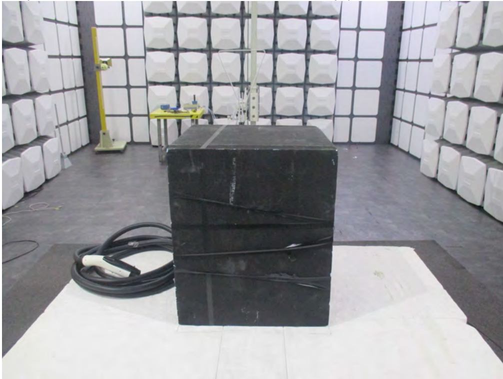
Description: Front View of Radiated Emission Test Setup (30 MHz ~ 1 GHz)
