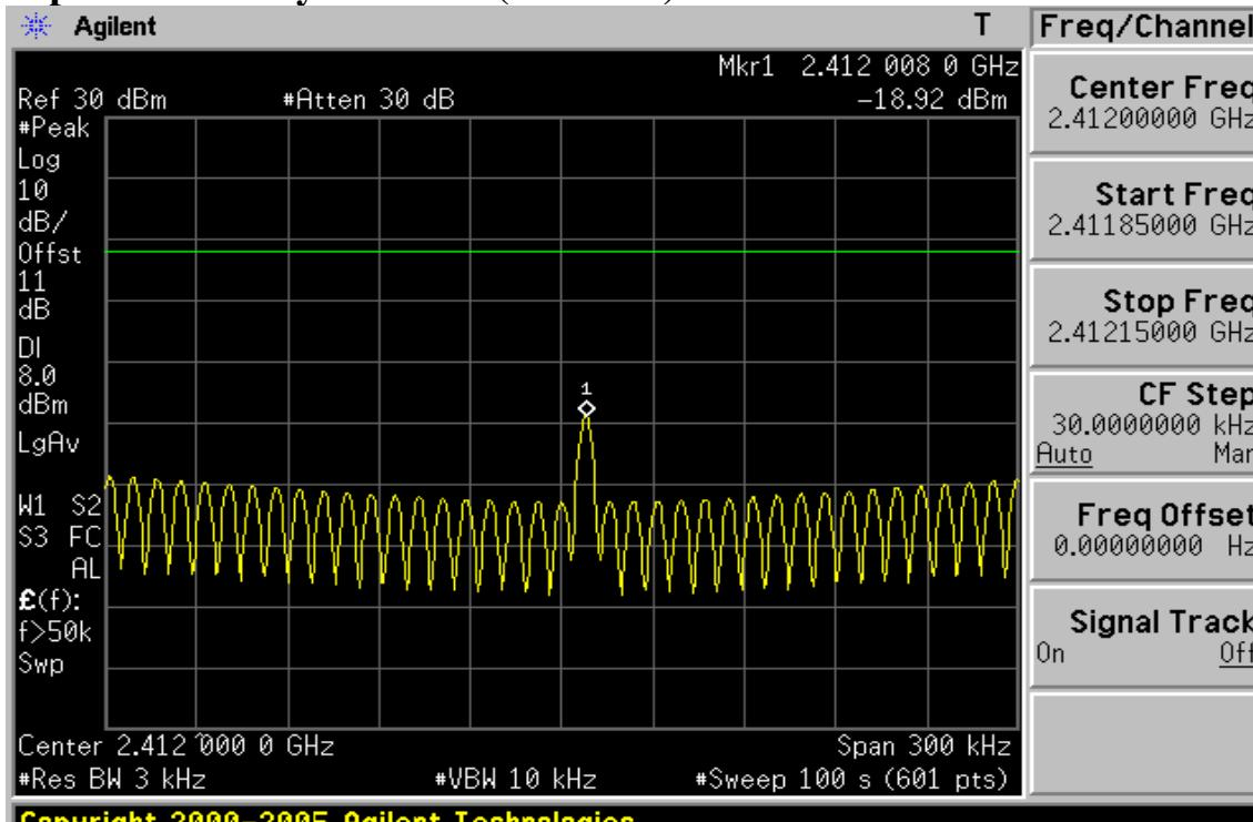
**Power Spectral Density Test Plot (CH-Mid)**
