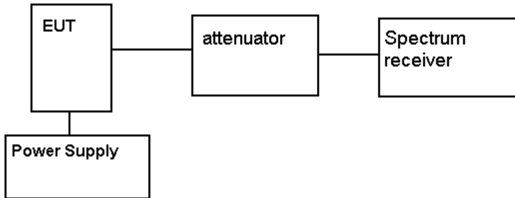
**METHOD OF MEASUREMENT:** The procedure used was ANSI/TIA 603-C:2004. The measurements were made at TIMCO ENGINEERING INC. 849 N.W. State Road 45, Newberry, Florida 32669.
