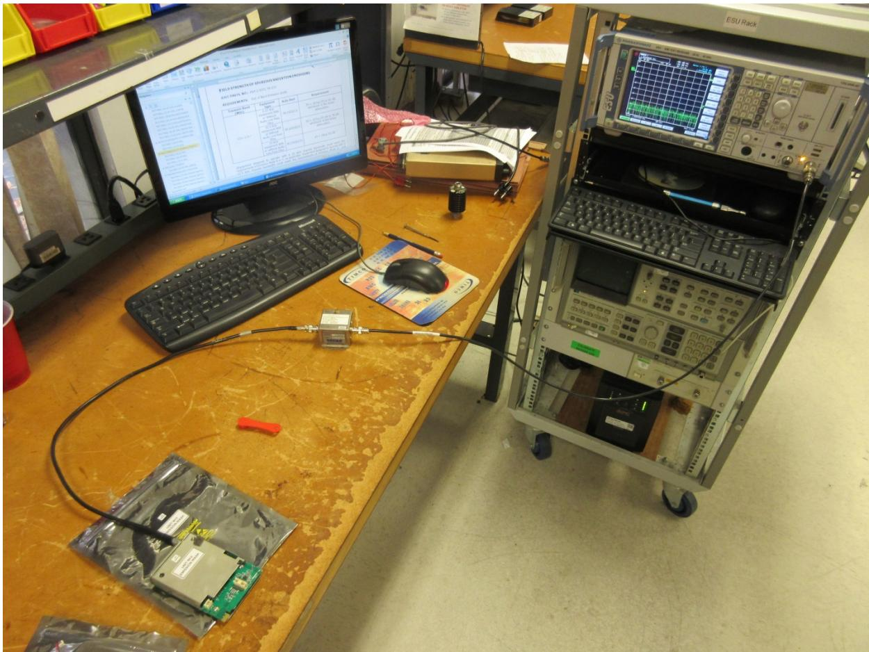
**FIELD STRENGTH SPURIOUS EMISSIONS FINAL EUT SETUP**
