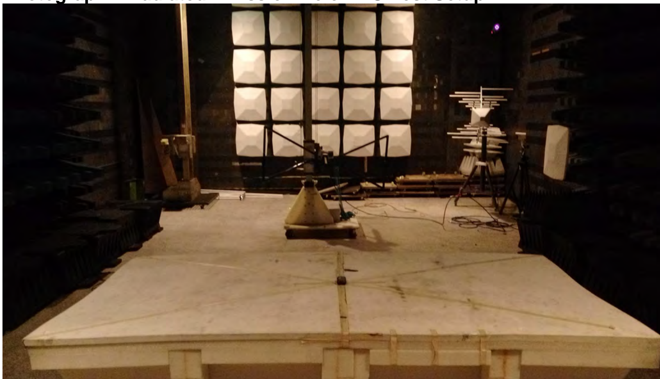
Photograph – Radiated Emission Below 1G Test Setup
