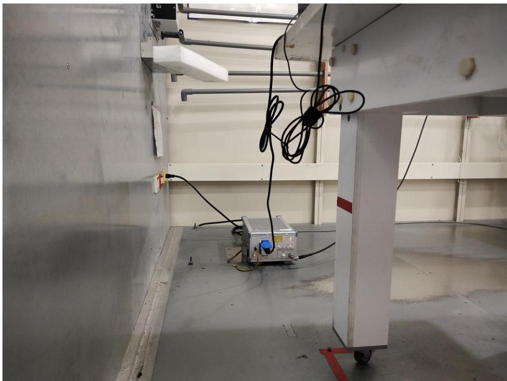
**Radiated emissions test photos****9 kHz to 30 MHz**
