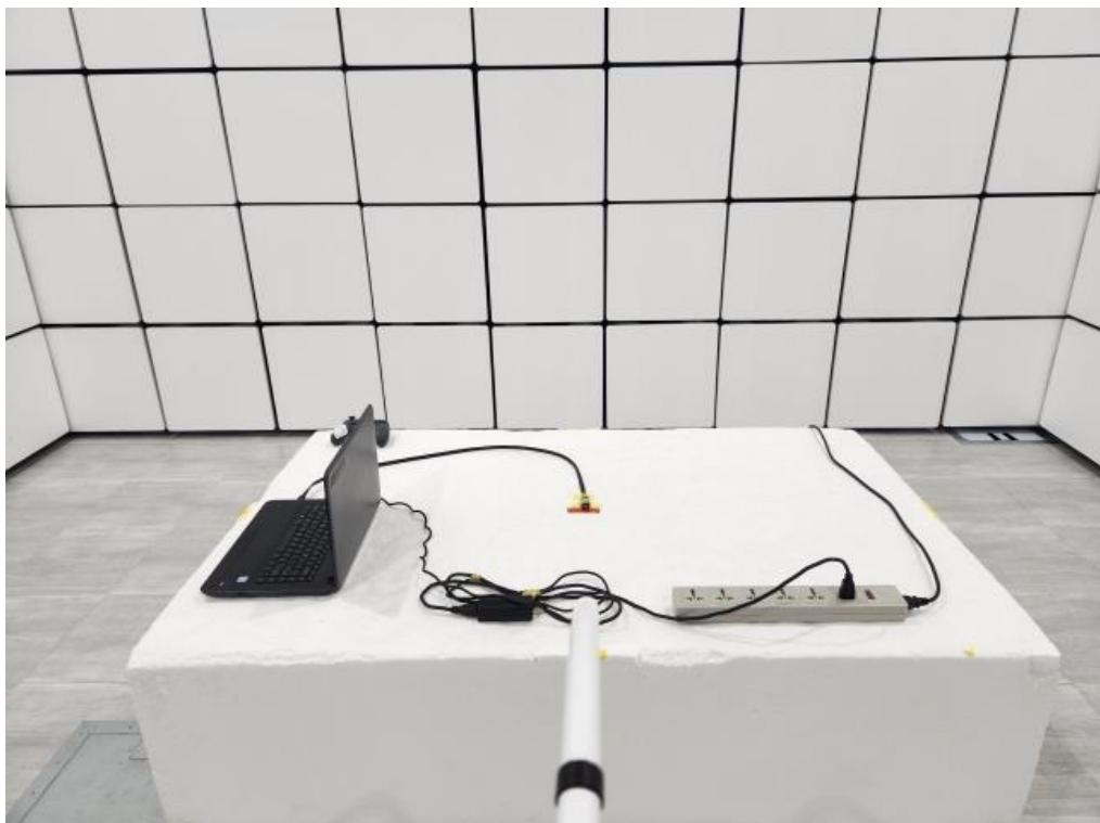
**Radiated emissions test photos****30 MHz to 1 GHz**
