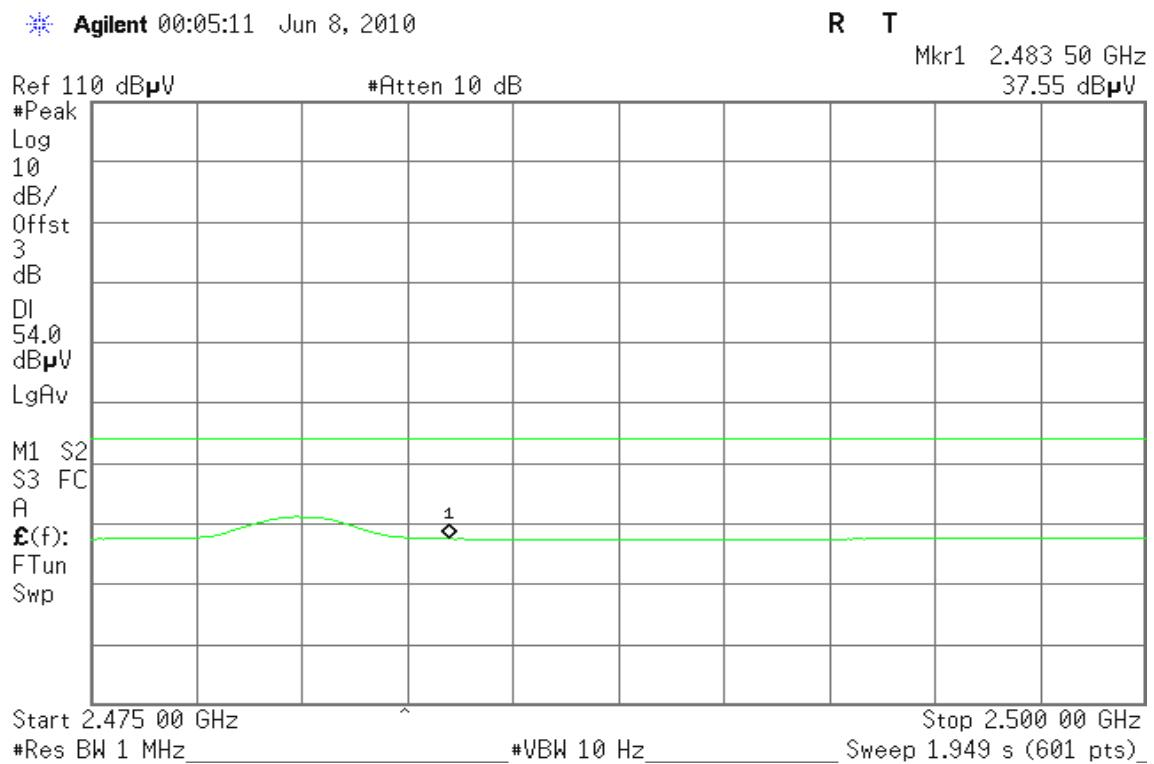
**Detector mode: Peak****Polarity: Horizontal**
