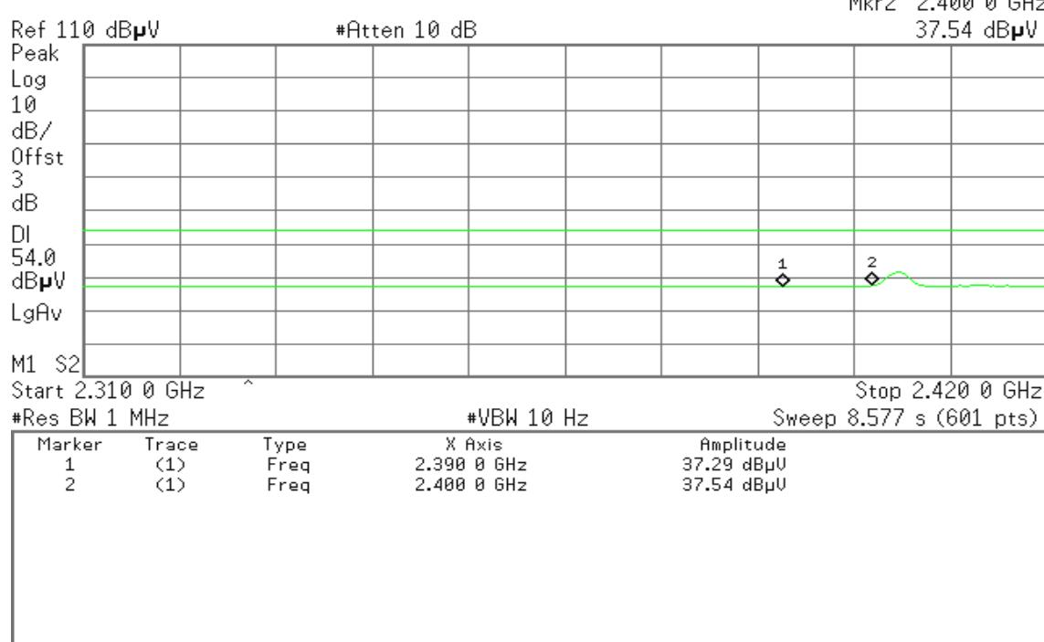
**Band Edges (CH High)****Detector mode: Peak****Polarity: Vertical**
