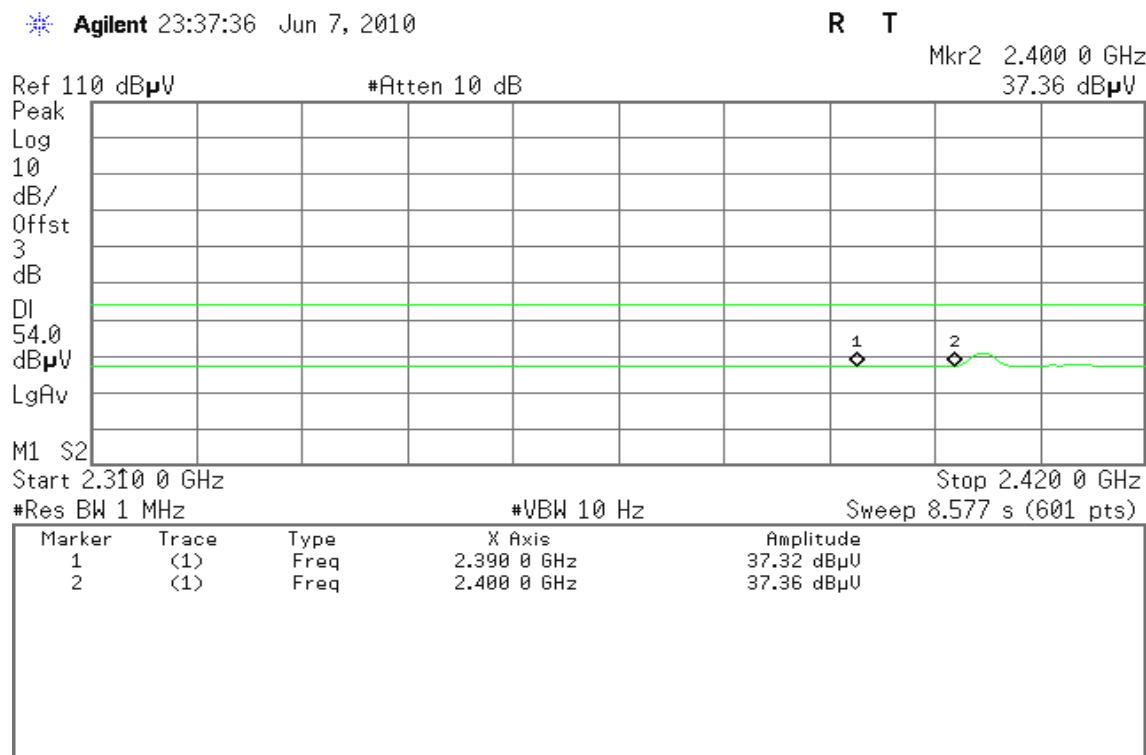
**Detector mode: Peak****Polarity: Horizontal**
