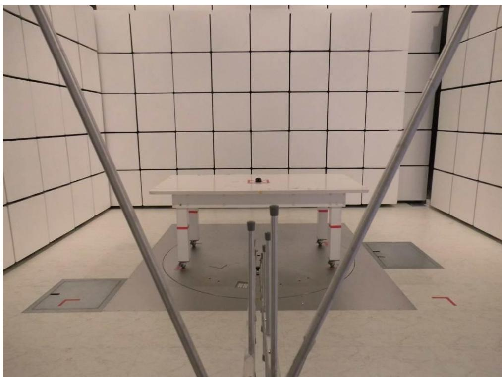
**Transmitter Radiated Emissions Test Photos****Above 1000 MHz**
