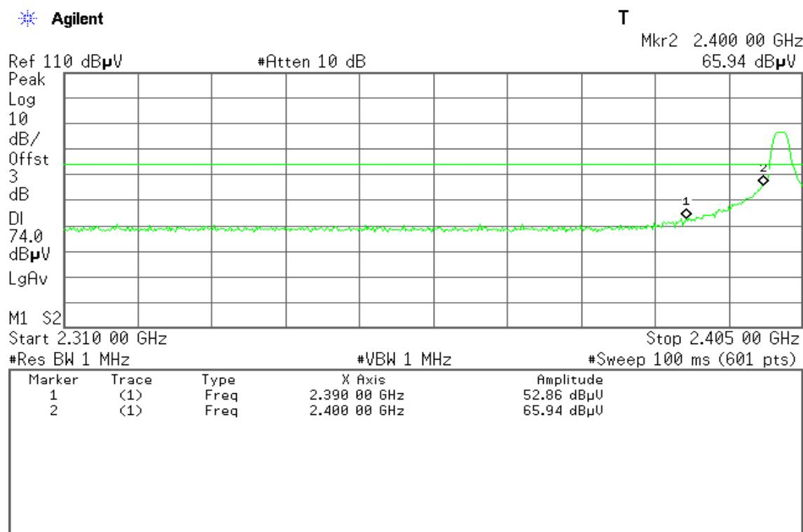
**Detector mode: Average****Polarity: Vertical**
