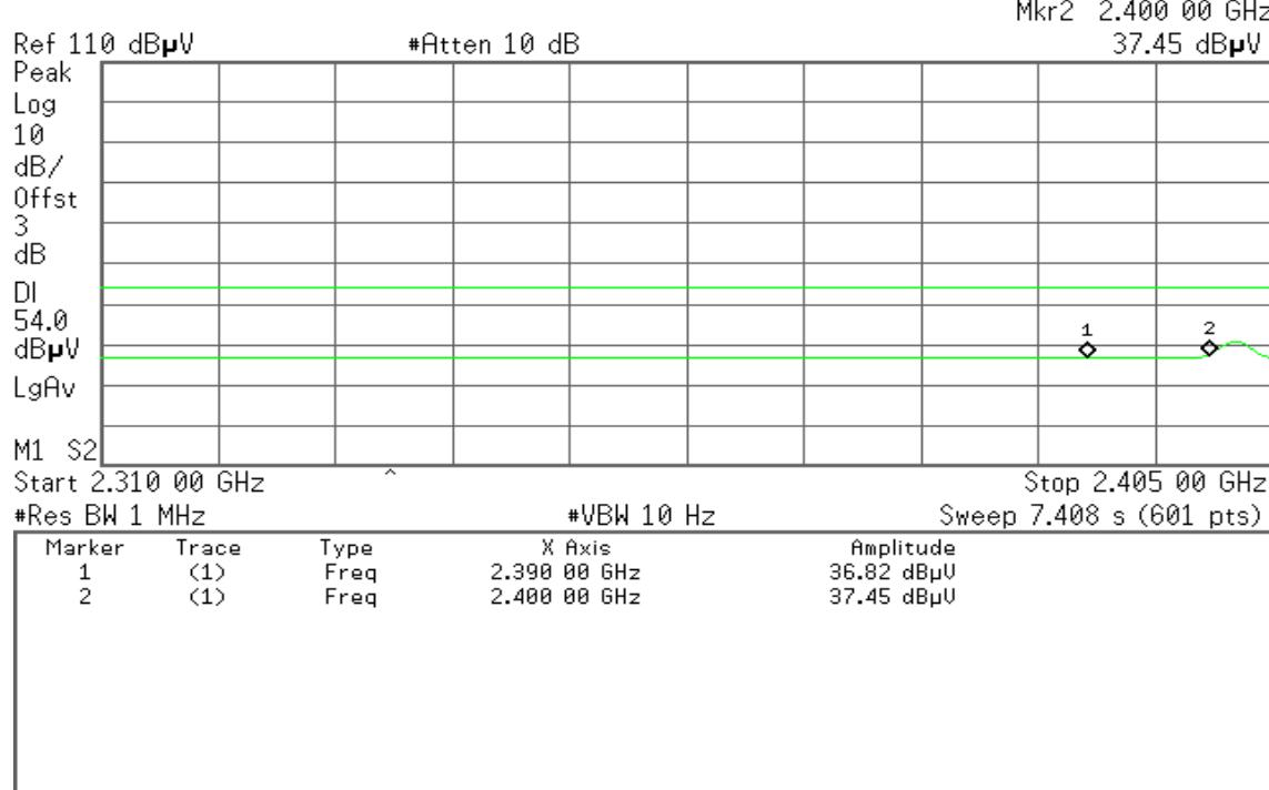
**Band Edges (CH High)****Detector mode: Peak****Polarity: Vertical**
