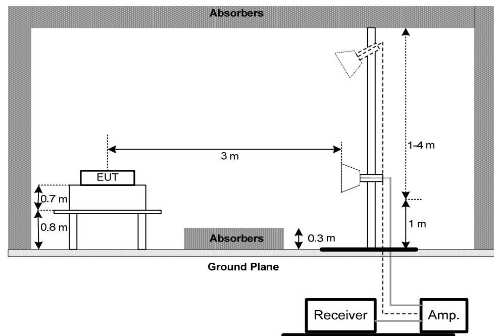
(C) For radiated emissions below 30MHz
