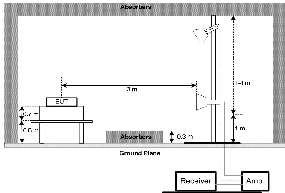
(C) For radiated emissions below 30MHz
