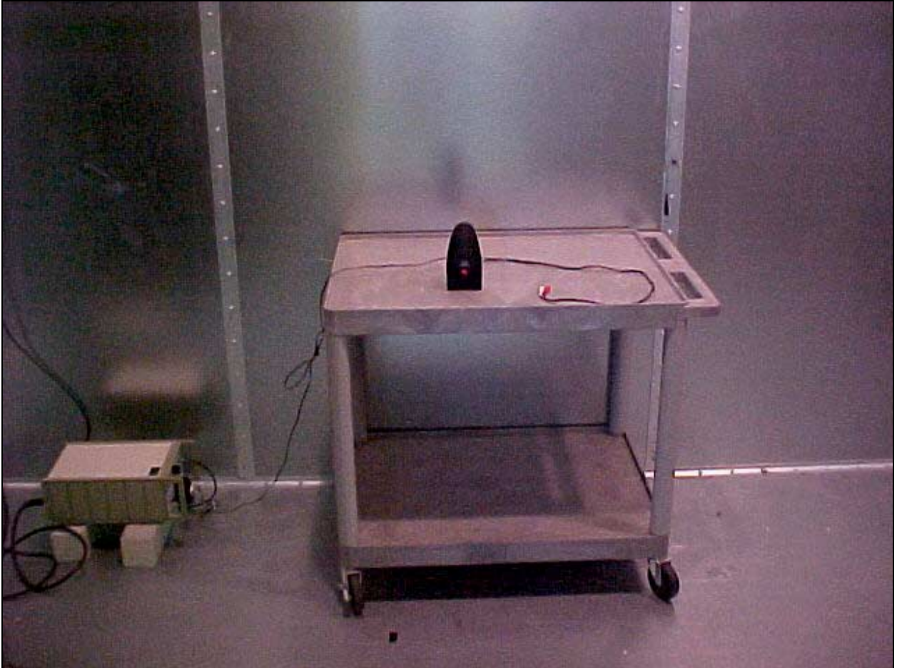
View of the EUT during Conducted Emissions Testing
