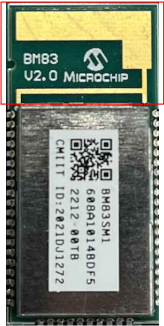
Inductor (RFID) :used as an antenna
