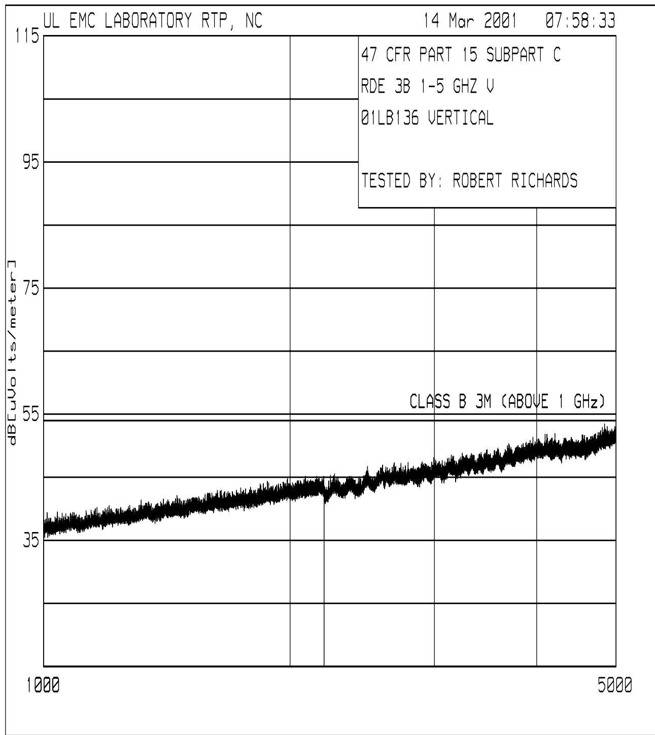
**Test 3, Item B (Idle) - Peak Plot (Amplitude in dBuV/m):**
