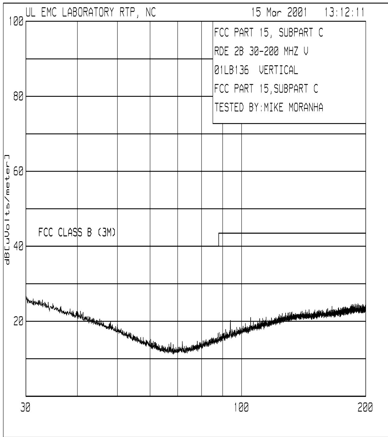
**Test 2, Item B (Idle) - Peak Plot (Amplitude in dBuV/m):**
