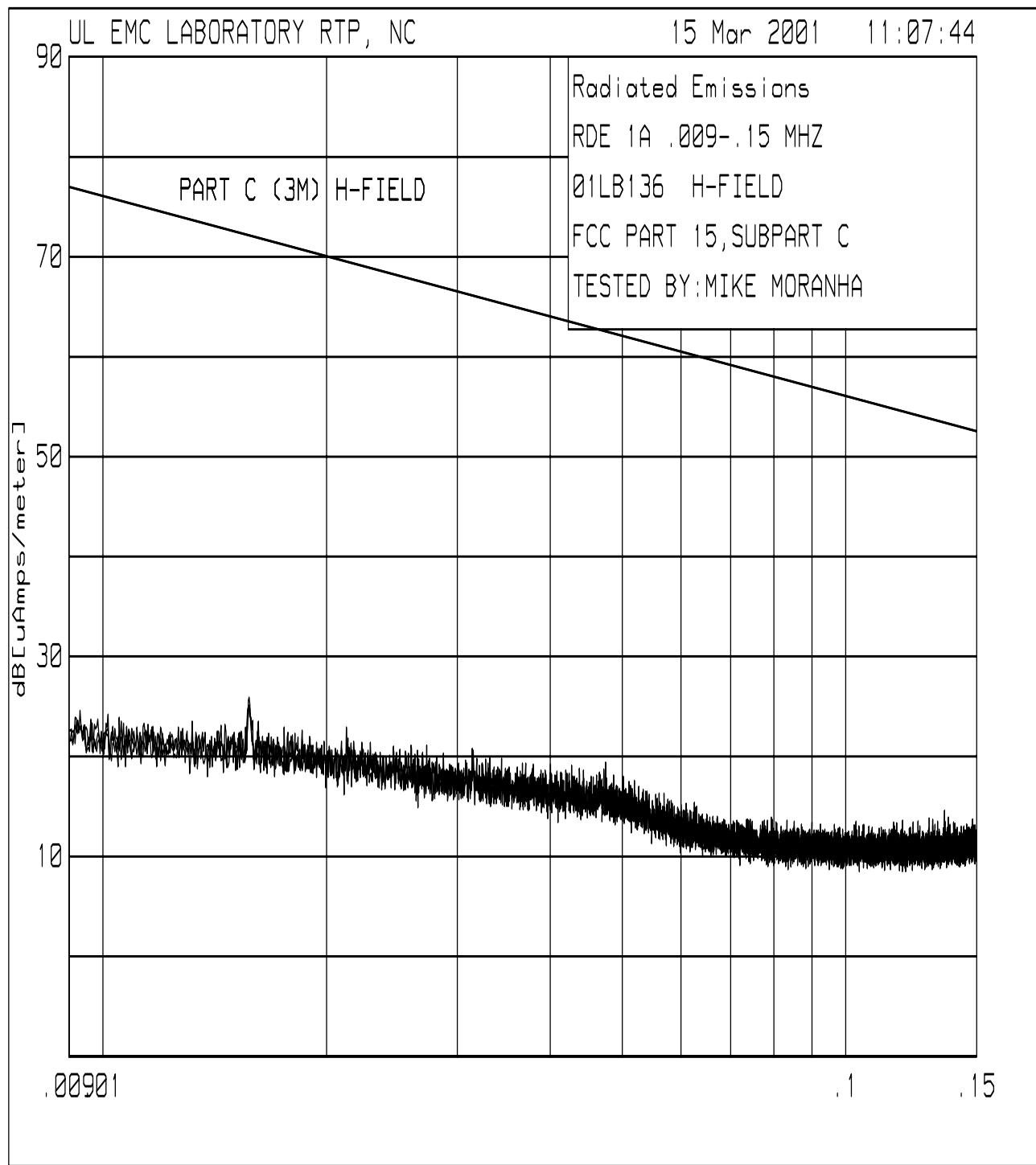
**Test 1, Item A (Transmit) - Peak Plot (Amplitude in dBuA/m):**
