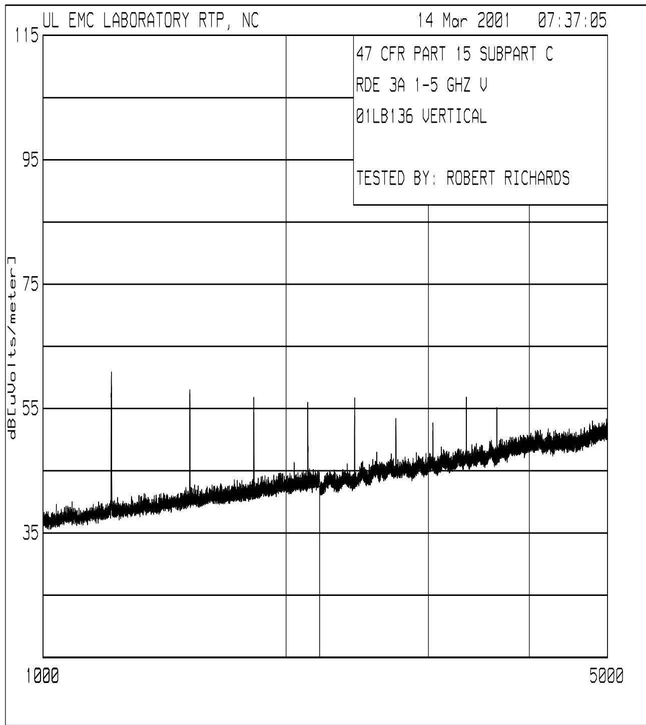
**Test 3, Item A (Transmit) - Peak Plot (Amplitude in dBuV/m):**
