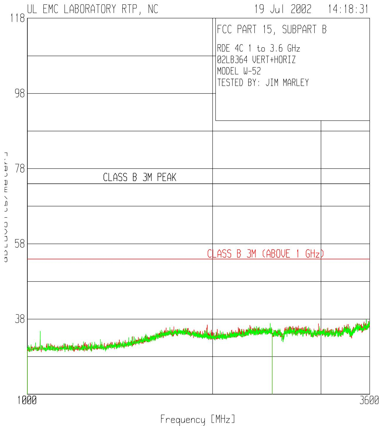
**Test 3, Item A - Discrete Data:****Radiated Disturbance Emissions - Above 1 GHz**
