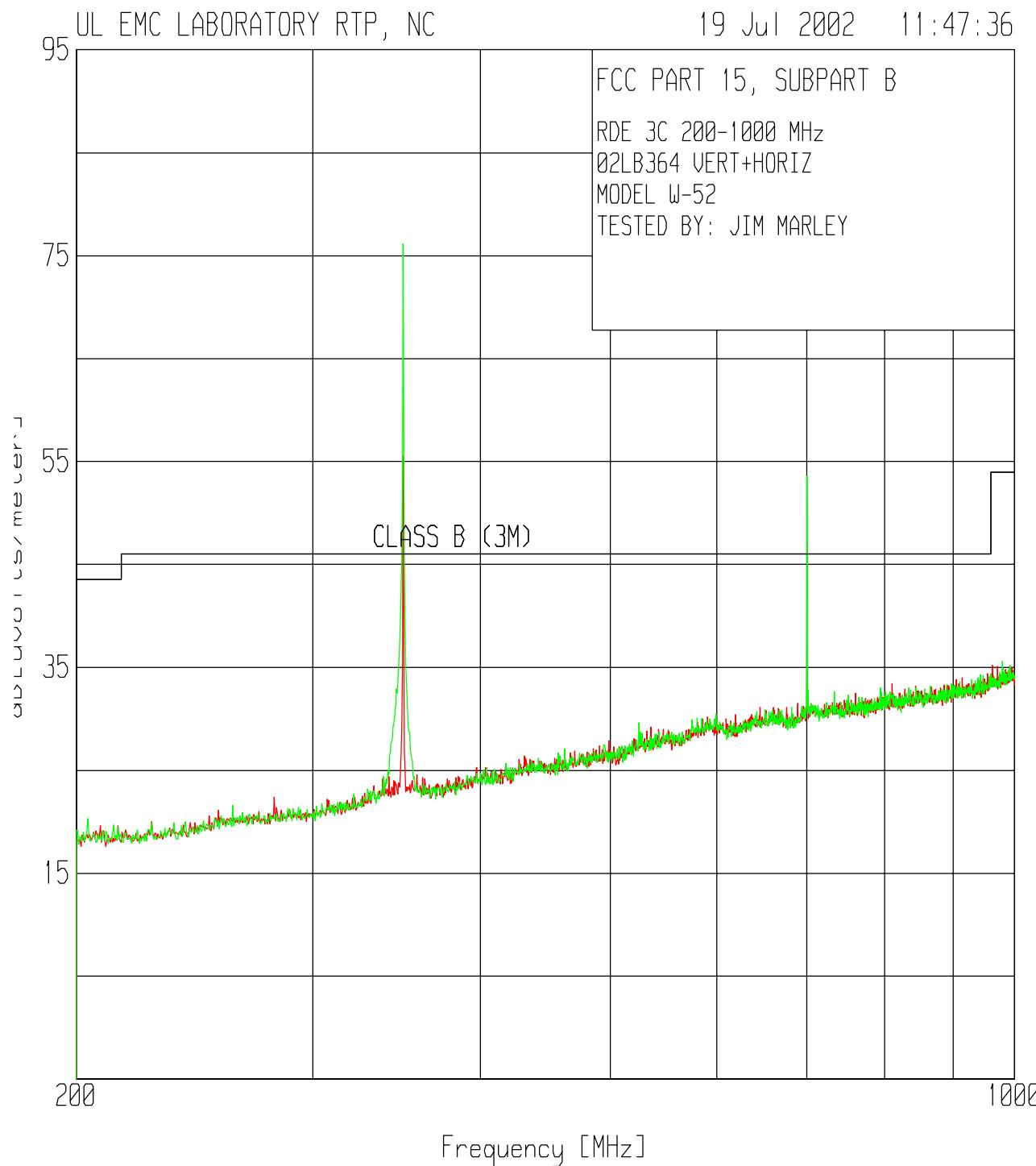
**Test 2, Item B (Idle, Not Transmitting) - Peak Plot (Amplitude in dBuV/m):**
