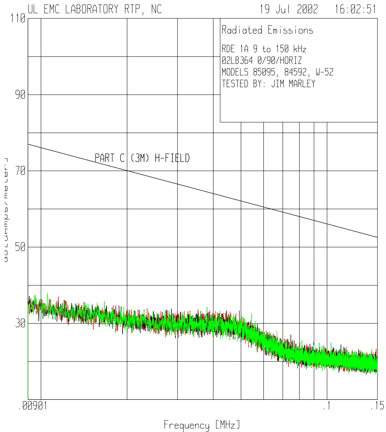
**Test 1, Item A (Transmitting) - Peak Plot (Amplitude in dBuV/m):**
