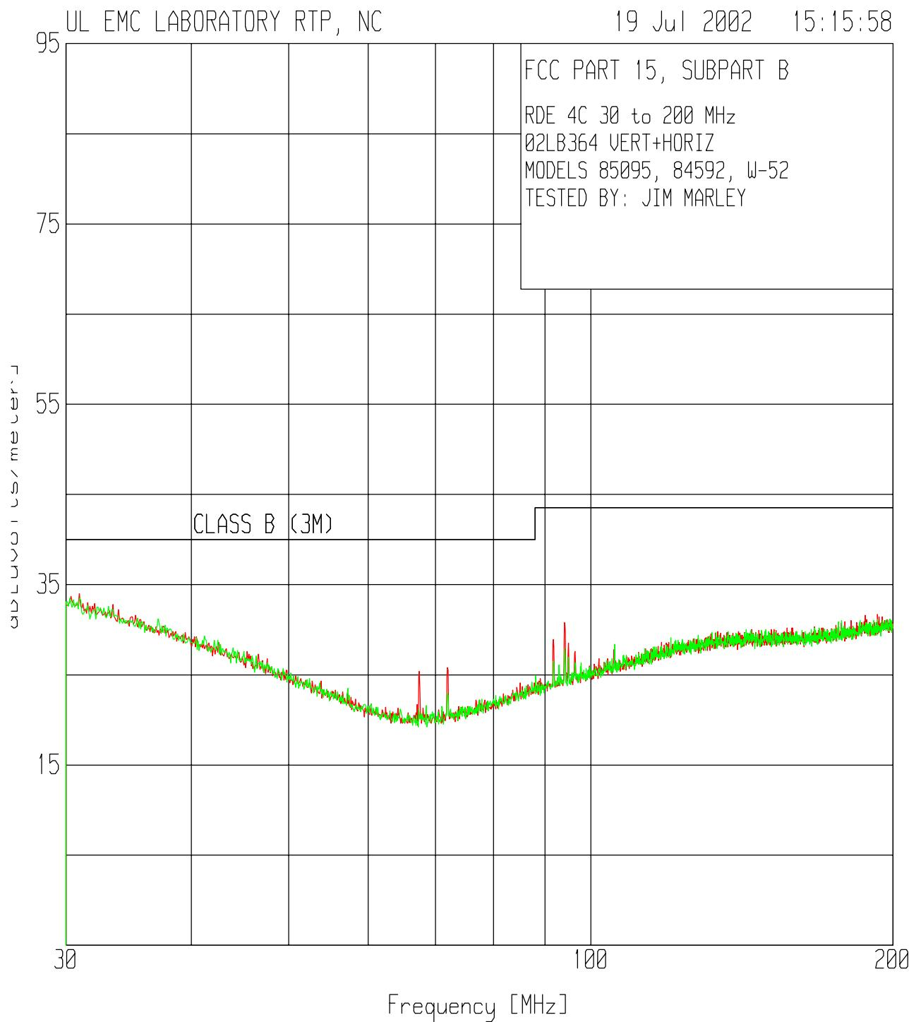
**Test 2, Item A (Transmitting) - Peak Plot (Amplitude in dBuV/m):**
