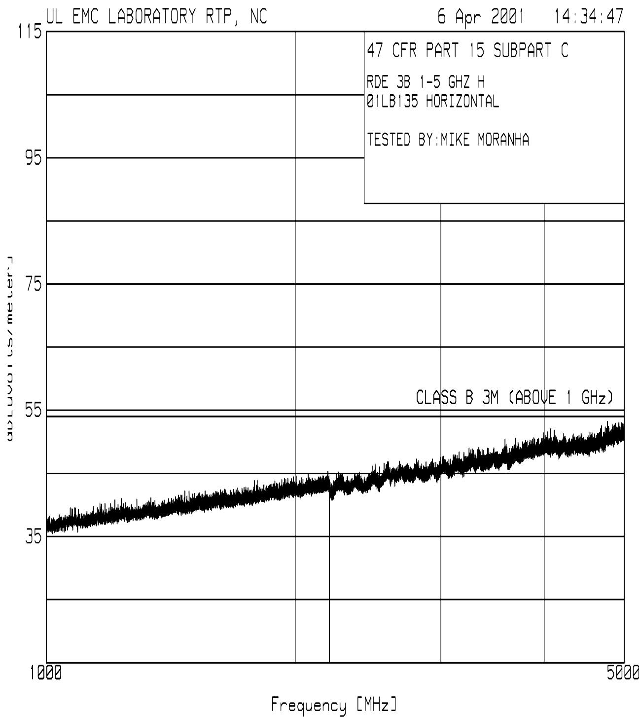
**Test 3, Item A (Transmit) - Discrete Data:** Radiated Disturbance Emissions - Above 1 GHz
