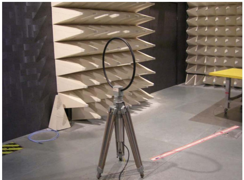
For radiated emissions 30MHz~1GHz
