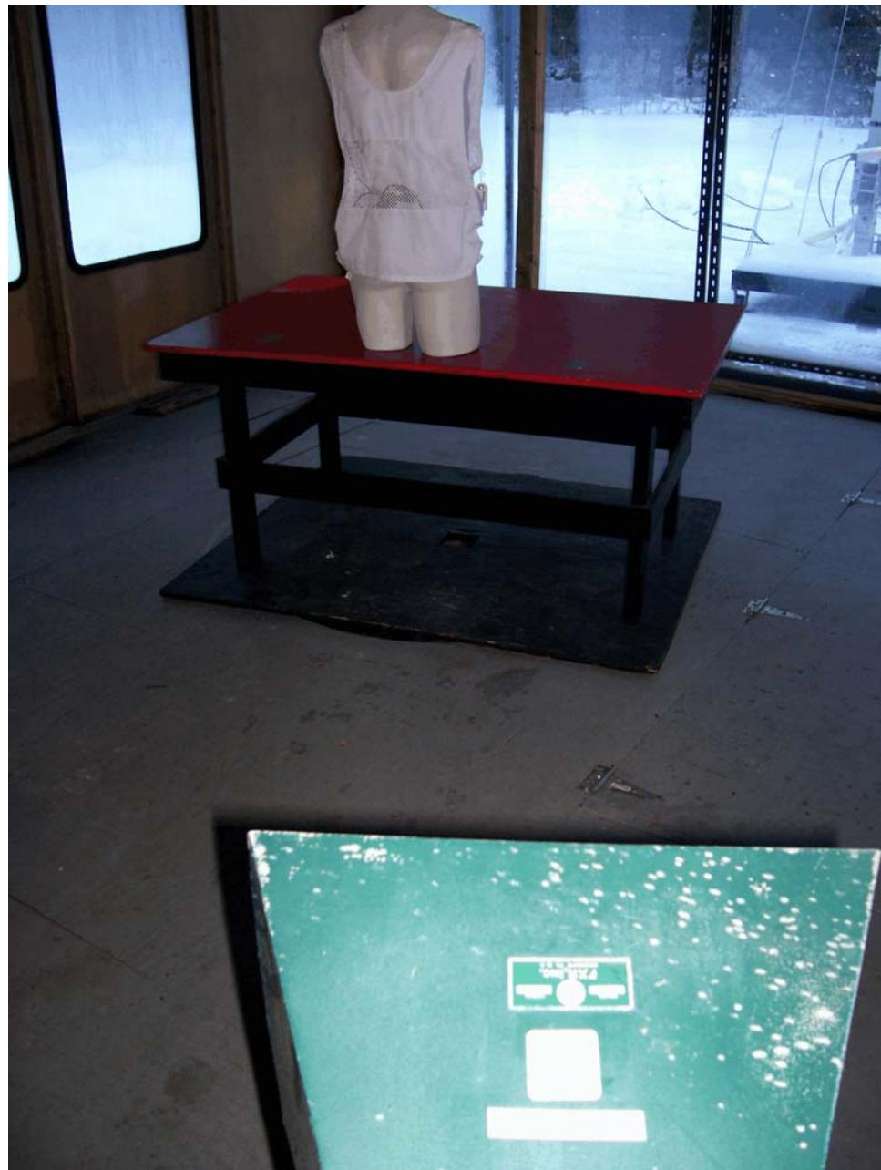
NOTE: The test sample was installed in the vest configuration in order to emulate the orientation and cable arrangement of how the device will be used in the field.
