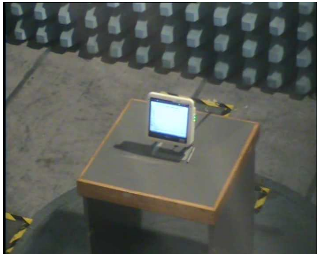
PHOTO 4 – SET-UP FOR EMISSION RADIATED TEST
