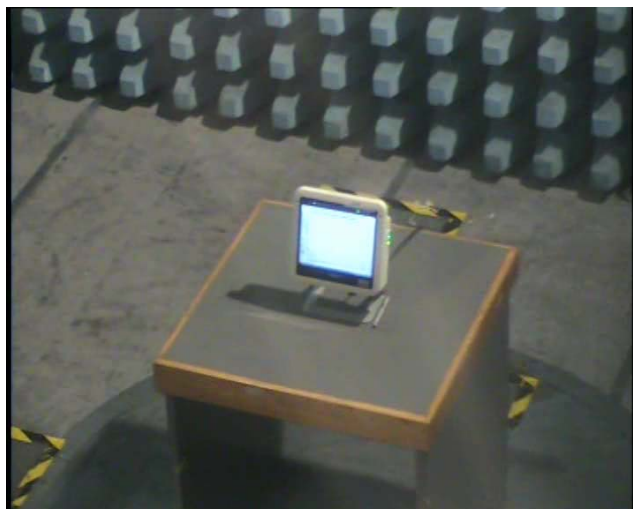
PHOTO 4 – SET-UP FOR EMISSION RADIATED TEST
