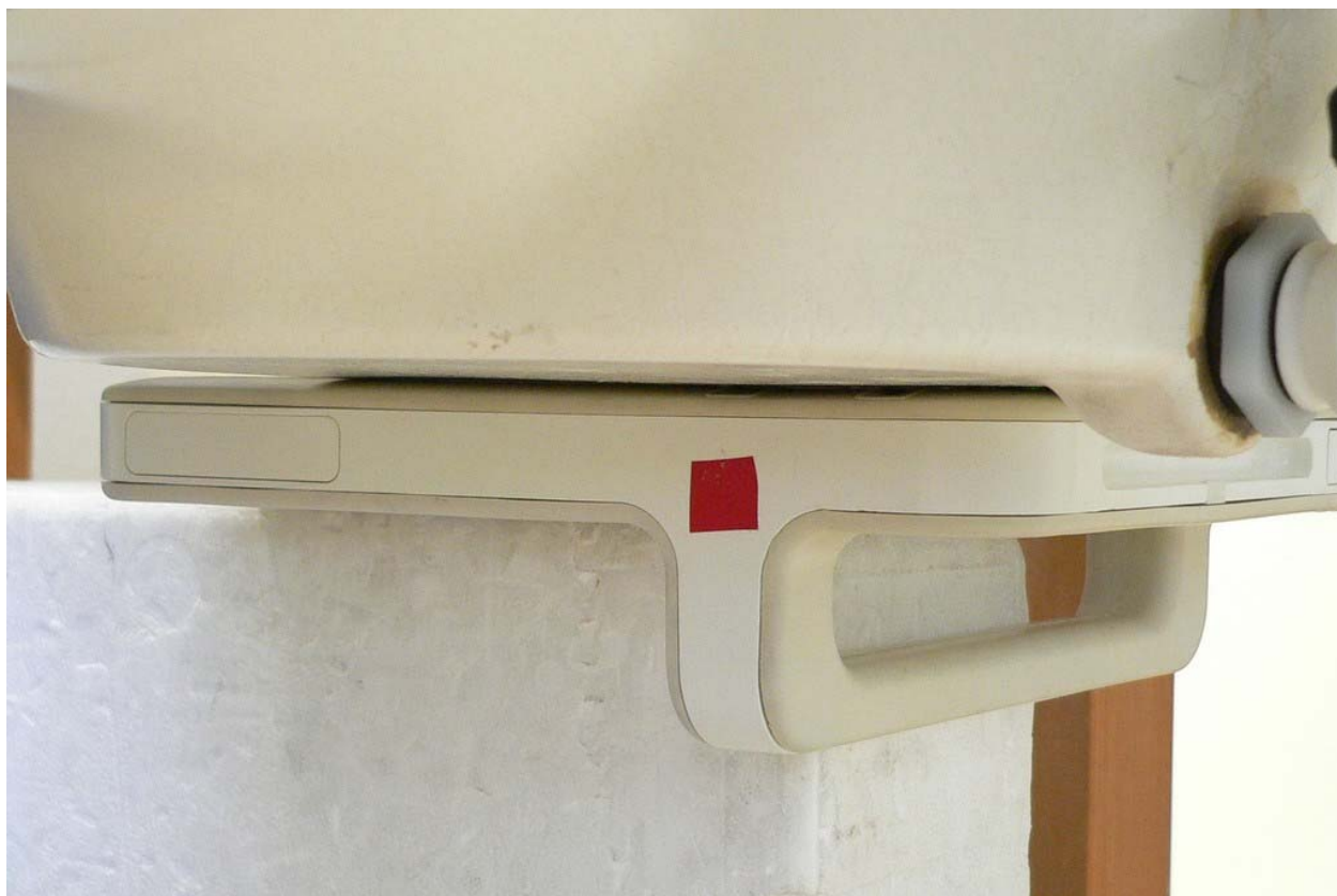
Fig. 19: Tested position for Antenna A worst case configuration, display touching the phantom.
