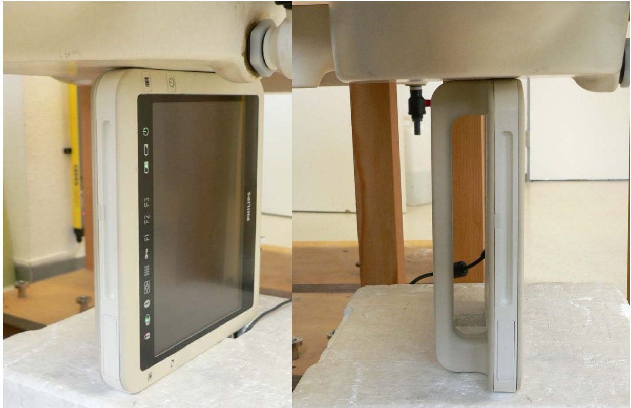
Fig. 17: Tested position for Antenna A, right side edge of the device.
