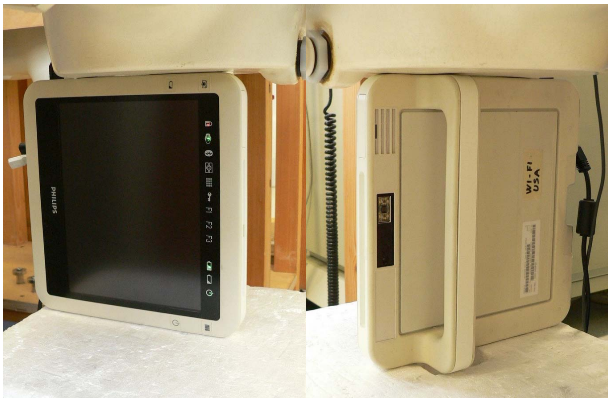
Fig. 18: Tested position for Antenna B, left side edge of the device.
