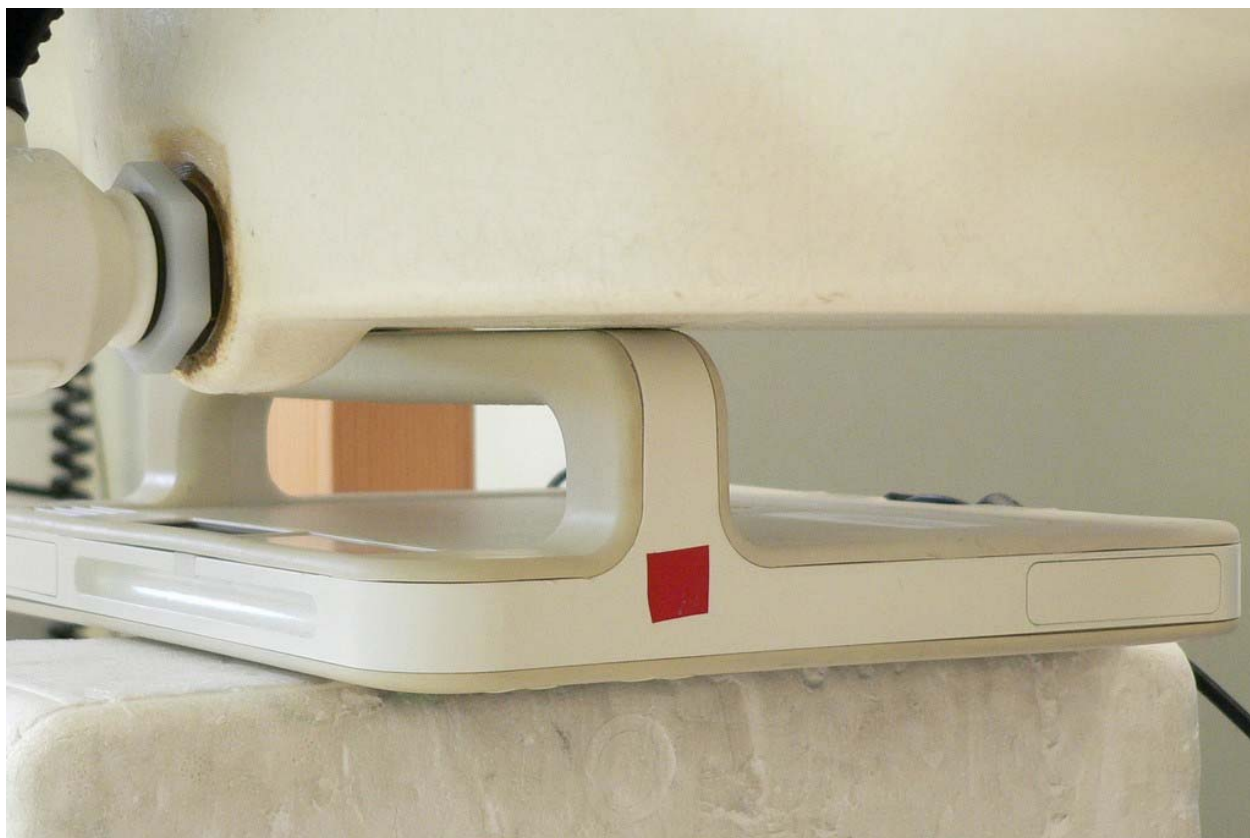
Fig. 20: Tested position for Antenna A worst case configuration, back side touching the phantom.
