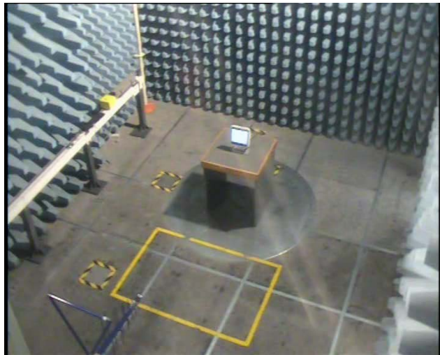
PHOTO 4 – SET-UP FOR EMISSION RADIATED TEST
