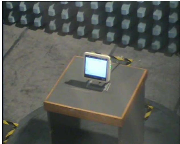
PHOTO 4 – SET-UP FOR EMISSION RADIATED TEST
