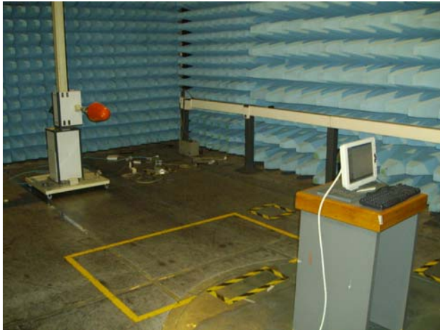
PHOTO 2 – SET-UP FOR EMISSION RADIATED TEST
