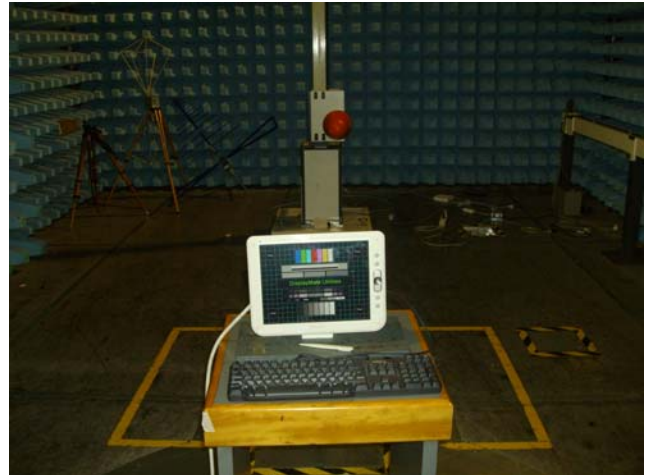
PHOTO 2 – SET-UP FOR EMISSION RADIATED TEST
