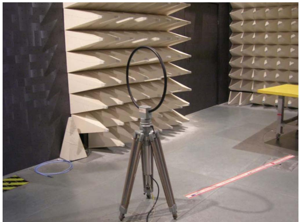
For radiated emissions 30MHz~1GHz
