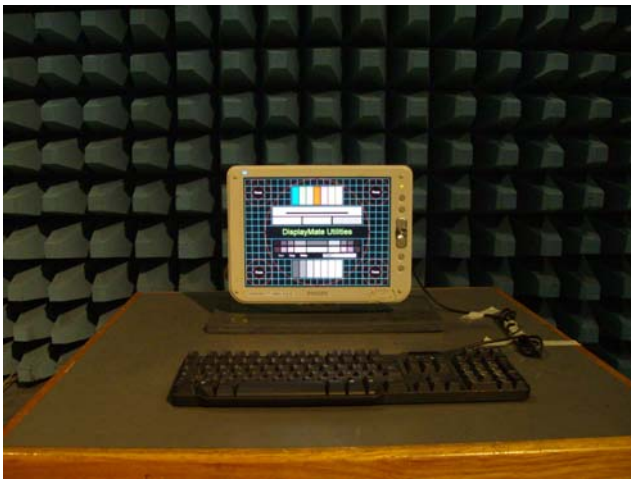
PHOTO N°1: Emission radiated setup with ancillary equipment
