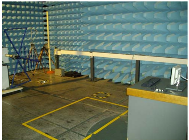
PHOTO N°1: Emission radiated setup with ancillary equipment
