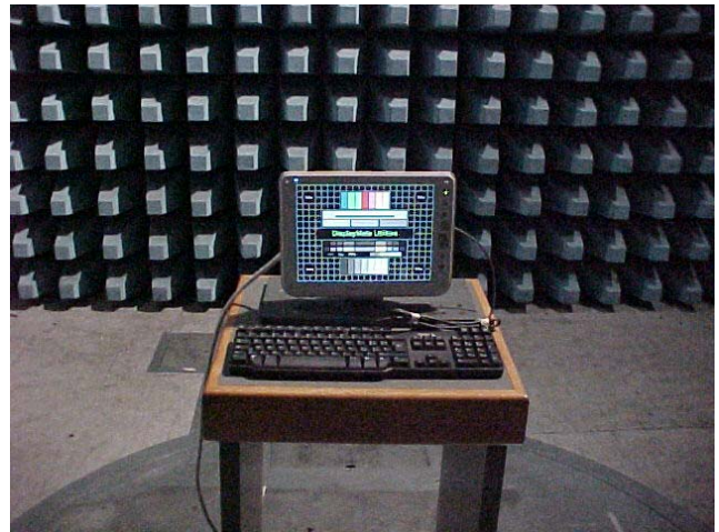
PHOTO 3 – SET-UP FOR EMISSION RADIATED TEST
