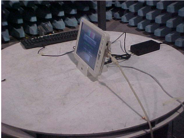
PHOTO 3 – SET-UP FOR EMISSION RADIATED TEST
