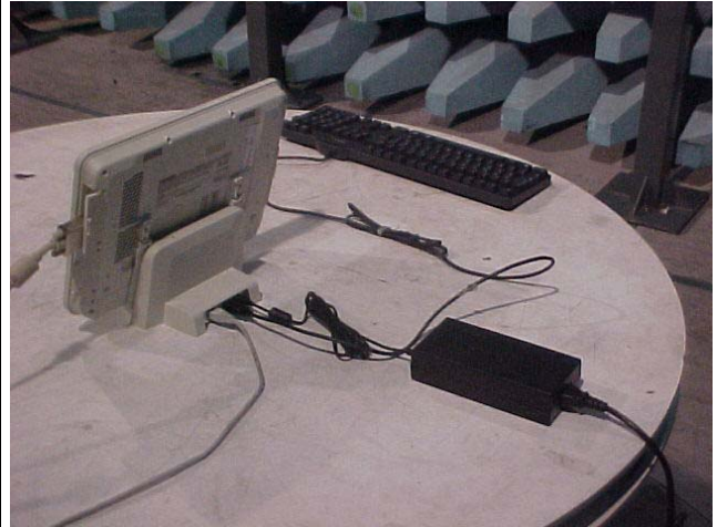
PHOTO 3 – SET-UP FOR EMISSION RADIATED TEST
