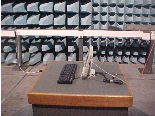
PHOTO 3 – SET-UP FOR EMISSION RADIATED TEST
