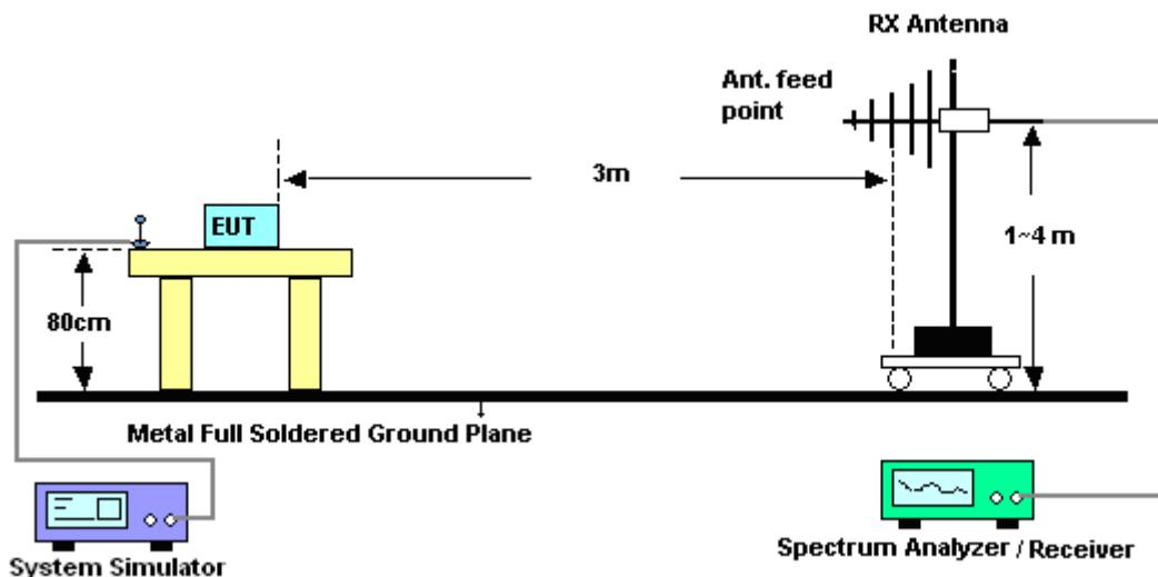
For radiated test above 1GHz
