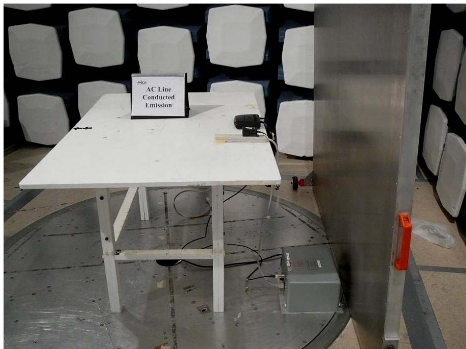
**14.3 Tx & Rx Spurious Radiated Emissions (Below 1 GHz) – Front View**
