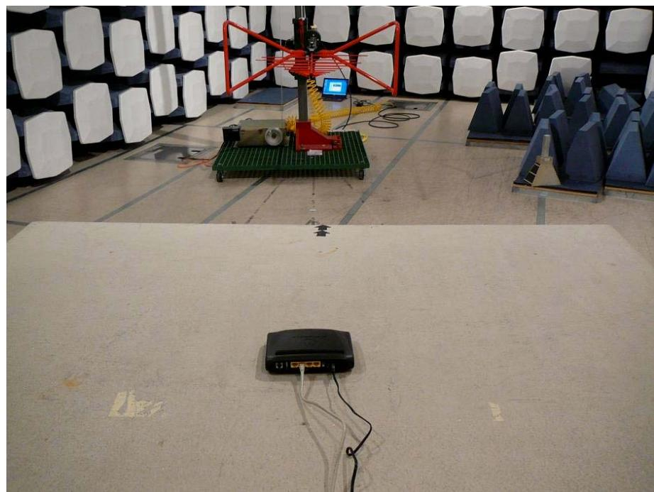
**14.5 Tx & Rx Spurious Radiated Emissions (Above 1 GHz) – Front View**
