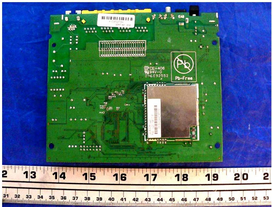
**EUT – Radio Card Detail View (RF Shielding Removed)**
