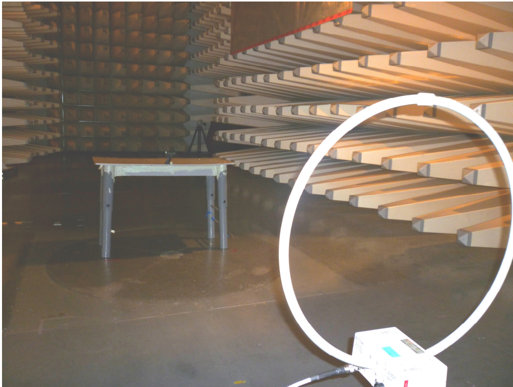
Set-up for Radiation Emission
