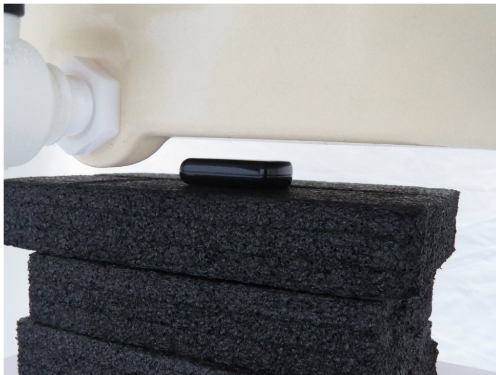
Picture 1: Back Side, the distance from EUT to the bottom of the Phantom is 10mm
