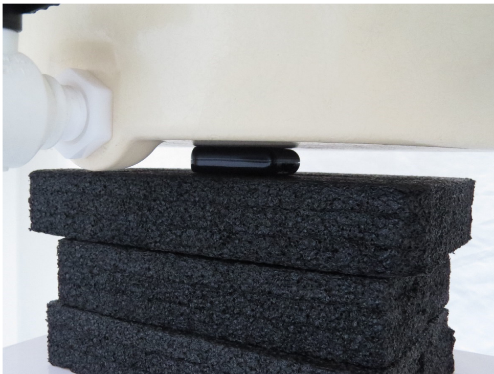
Picture 7: Front Side, the distance from EUT to the bottom of the Phantom is 0mm
