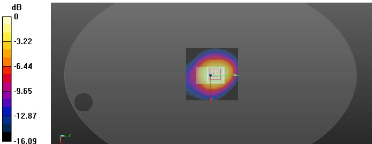
$$0 \text{ dB} = 0.422 \text{ W/kg} = -3.75 \text{ dBW/kg}$$
