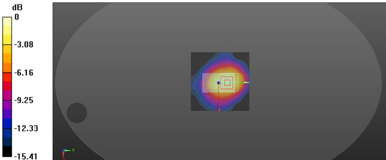
$$0 \text{ dB} = 0.124 \text{ W/kg} = -9.07 \text{ dBW/kg}$$
