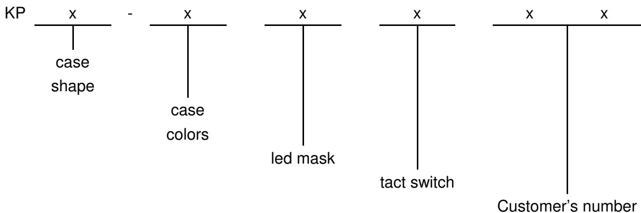
The case shape: such as right angle, concave, convex and special angle. The case shape will not influence PCB board.
