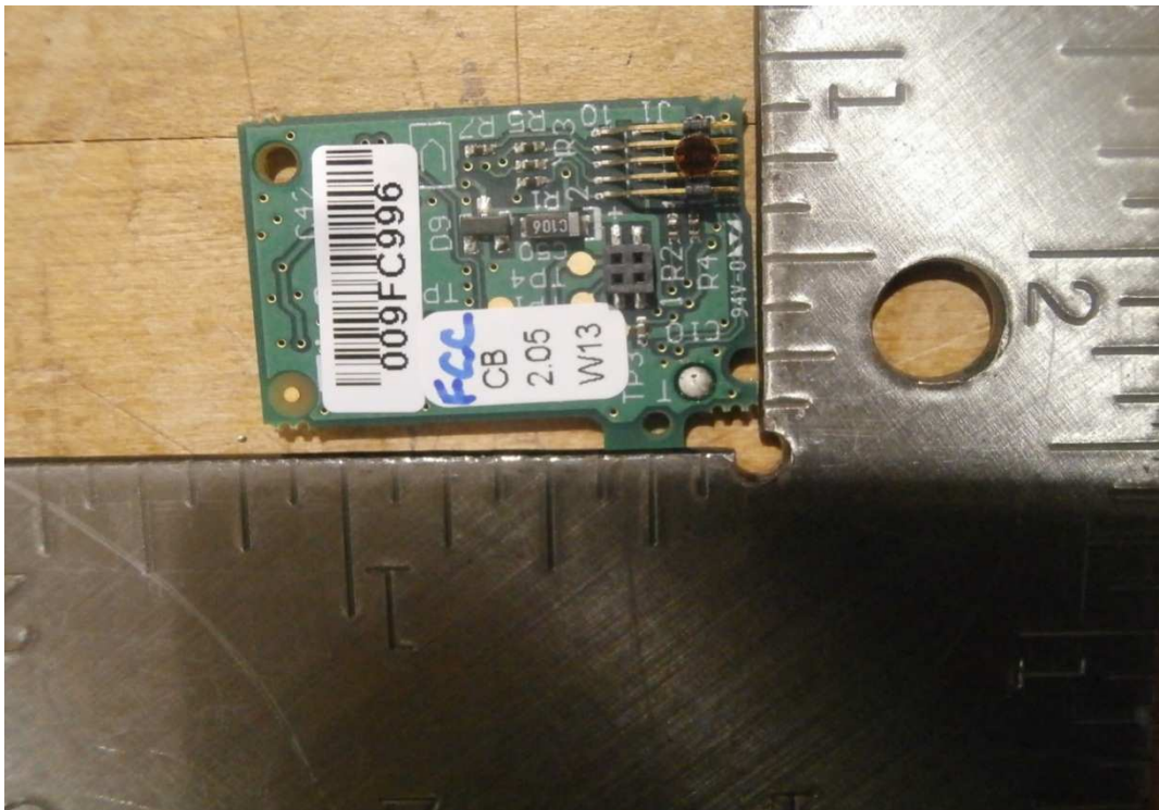
RF Board Bottom view
